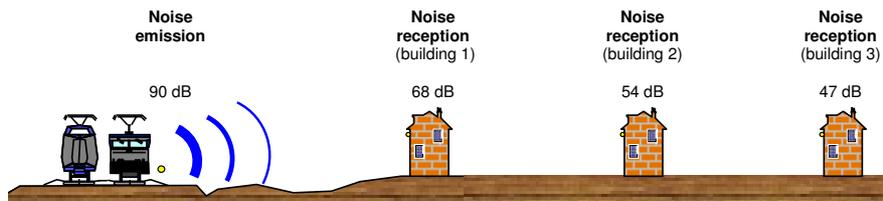
**Fig. 2.** Emission level and reception levels.
