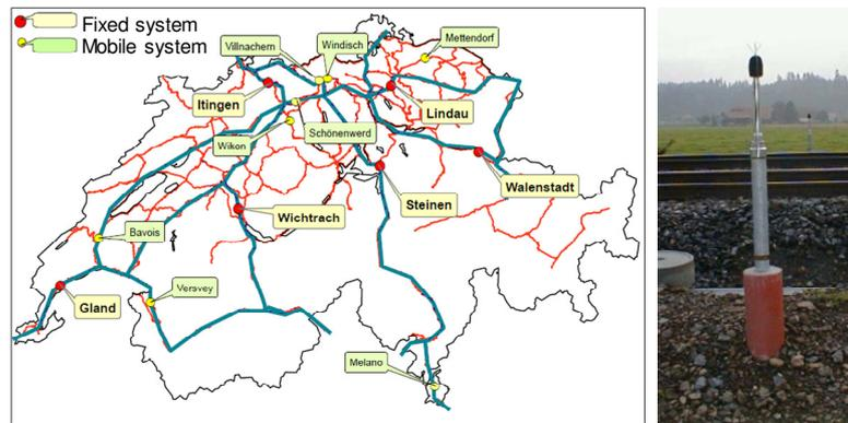
Fig. 3. Fixed and mobile measurement sites on the Swiss railway network.
