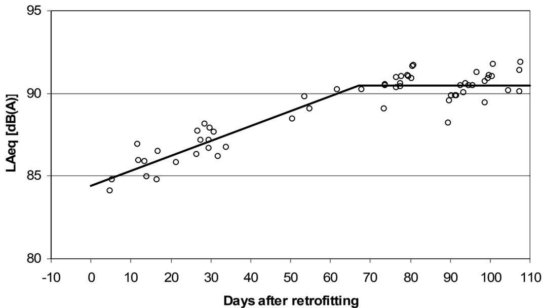
Fig. 4. Development of pass-by noise level after retrofitting and reprofiling.
