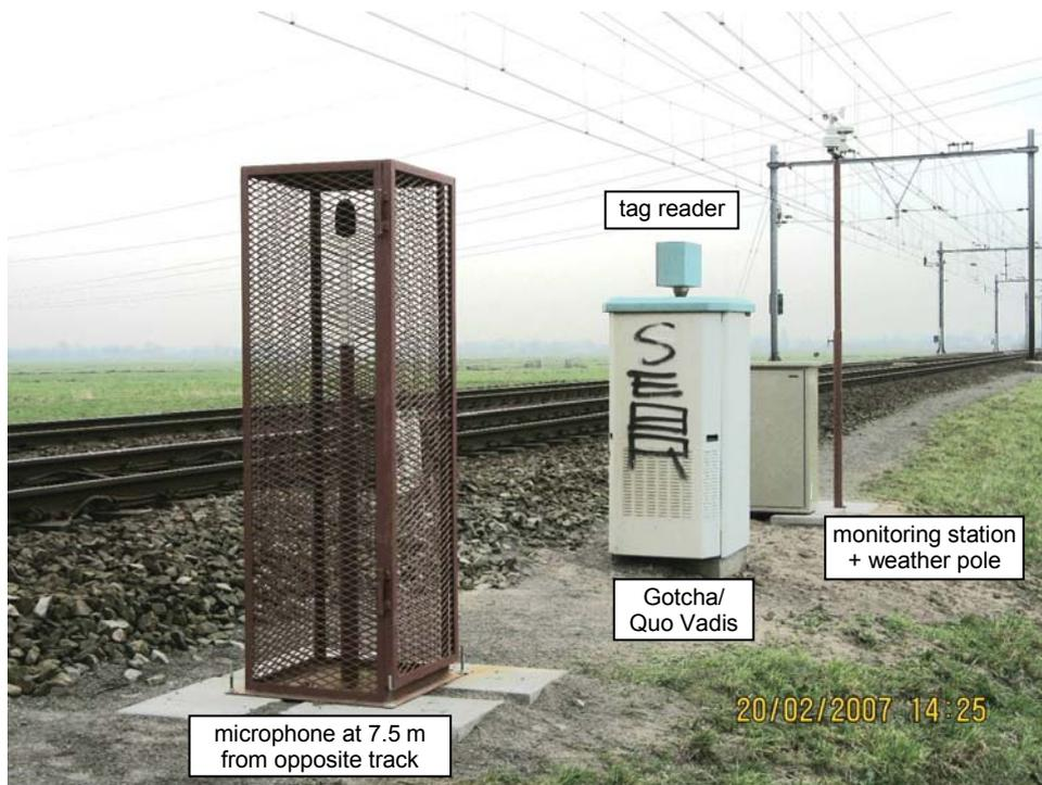
Fig. 1. Noise monitoring station along the railway track (line Weesp – Almere).
