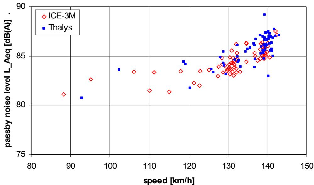
Fig. 6. A-weighted equivalent sound pressure level of high speed trains.
