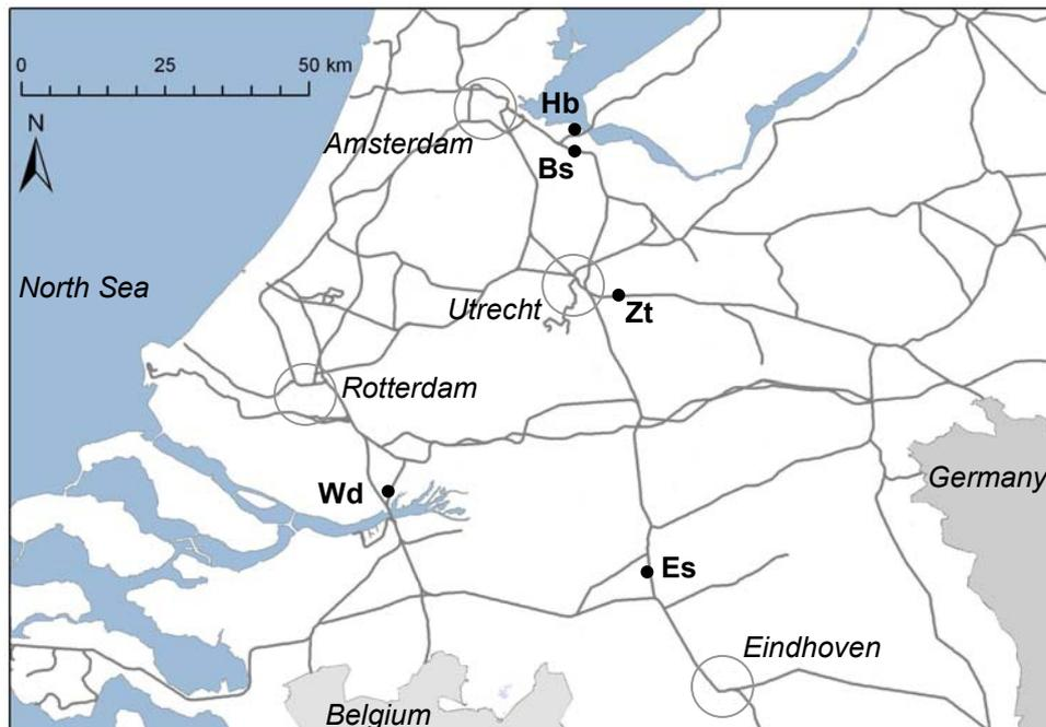
Fig. 2. Railway network and positions of noise monitoring stations (Wd, Es, Bs, Zt, Hb).
