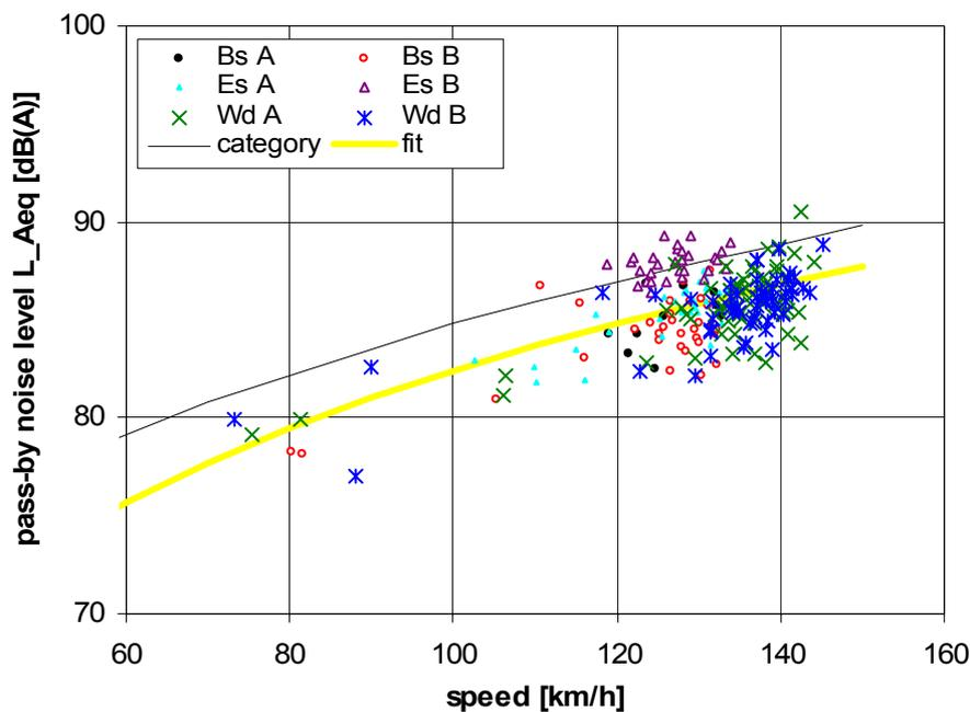
Fig. 4. A-weighted equivalent sound pressure level of IRM trains.
